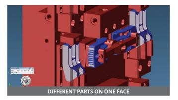
The ability to generate CNC code in single-part mode to prove set up and machining before running a fully loaded tombstone
