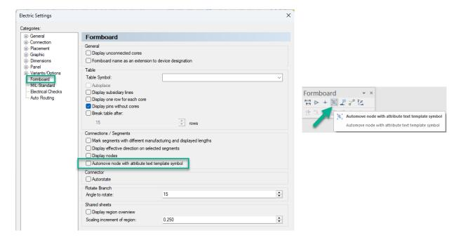
If the new setting is active, underlying nodes on the formboard net are also moved when attribute text template symbols are moved, provided these nodes are not fixed.
