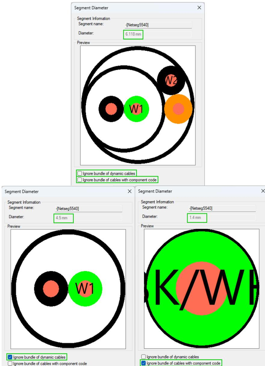
The settings **Ignore bundle of dynamic cables** and **Ignore bundle of cables with component code** can be activated and deactivated temporarily in order to compare the changes of segment diameters.
